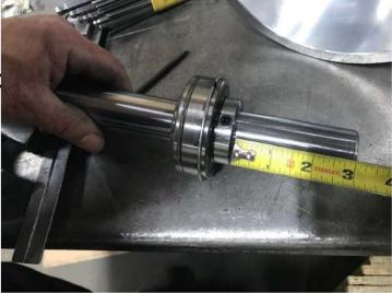
Be sure spindle is flush with pulley ID face.
