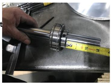
Be sure spindle is flush with pulley ID face.
