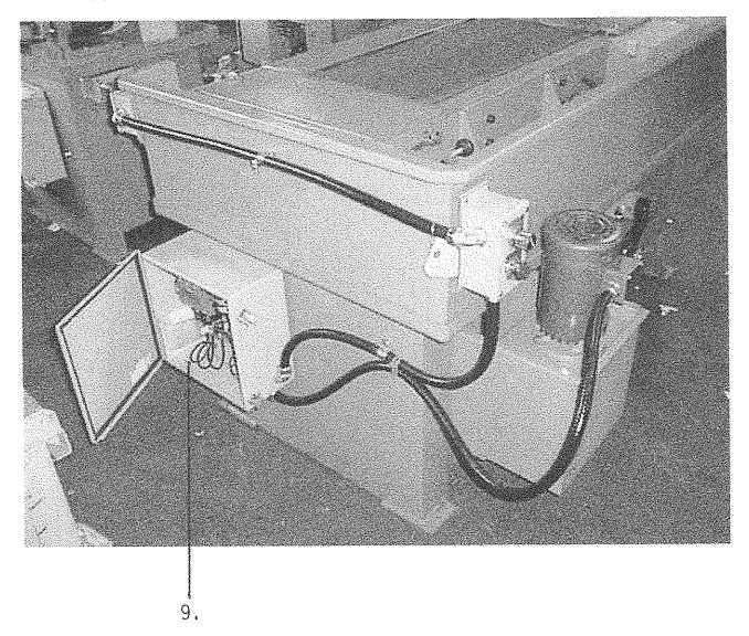
9. Power box- Houses magnetic starter, transformer, electronics. Bring user power into power box. Customer to drill holes and locate per customer standards. Use appropriate fittings per local codes etc..
