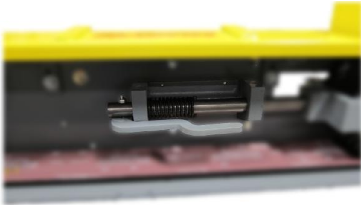
Spring belt tension (close-up)
