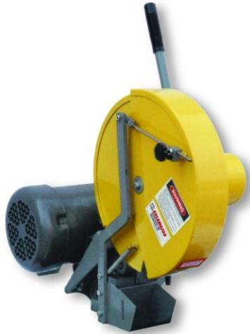
The HS14AS is a purpose-built high-speed saw engineered specifically for cutting non-ferrous metals. With a powerful 5HP motor driving the blade at 4,400 RPM, this saw delivers the speed needed for clean, burr-free cuts on aluminum, brass, copper, and other soft metals.
